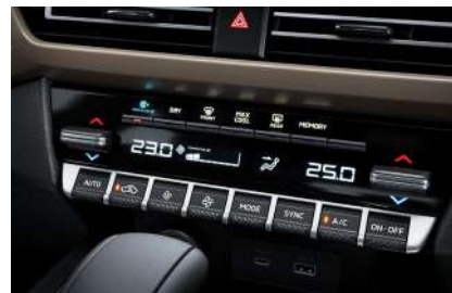
Dual-zone automatic air conditioning and rear air vent Temperature settings can be adjusted independently for the driver's seat, front passenger seat.
